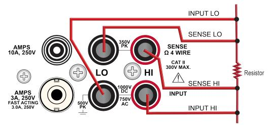
Figure 36: Rear-panel connections for 4-wire resistance measurements
