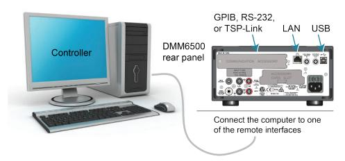
Figure 15: DMM6500 remote interface connections
