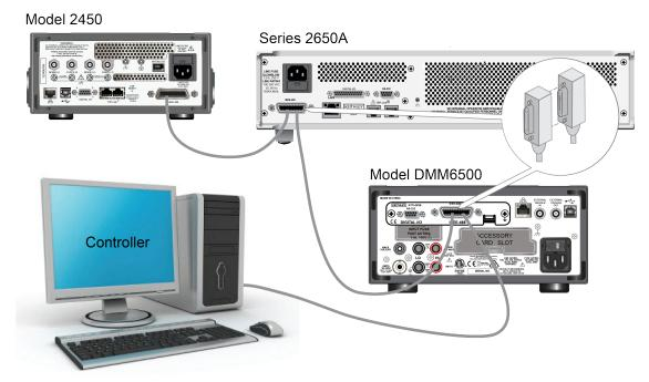
Figure 23: DMM6500 instrument GPIB connections
